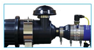
We install a state-of-the-art MPS gas sensor in the air intake system of the engine, that reads flammable gasses. Unlike Cat bead/Pellister type sensors, the MPS gas sensor calibrates itself every 2.0 seconds using up to date ambient temperature, barometric pressure, and relative humidity. It does not require bump gas, docking stations or an instrument technician to recalibrate 4 times a year.
