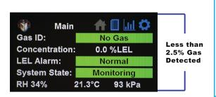
The data is also sent to the display, giving you a real time display of the sensors findings.
