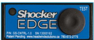
The sensor reads the chemical composition of the air being drawn into the engine, then transmits the data to the ShockerEDGE controller and the ShockerEDGE display.
